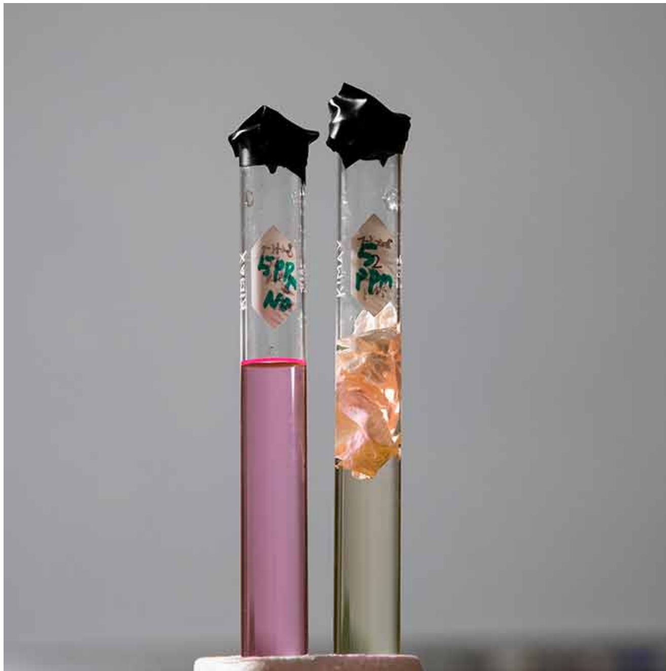
The tube on the left shows a red dye solution. In the tube on the right, the dye was trapped by a reusable web invented by a team at Texas Tech University. Light can then break down the dye. Texas Tech University
