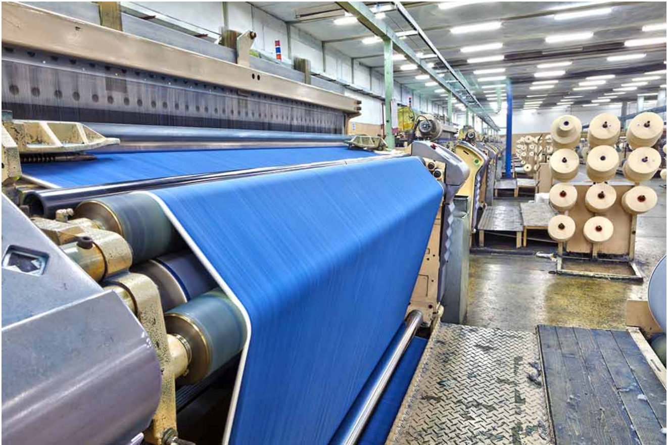
Dyed yarns are woven into denim on an air jet loom. danishkhan/E+/Getty Images Plus
