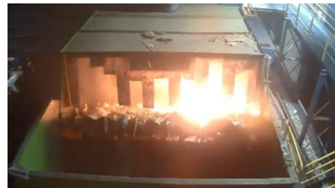
Picture: Fire started by battery improperly disposed in recycling at Shoreway Environmental Center Materials Recovery Facility costing the facility $6.8 million in
