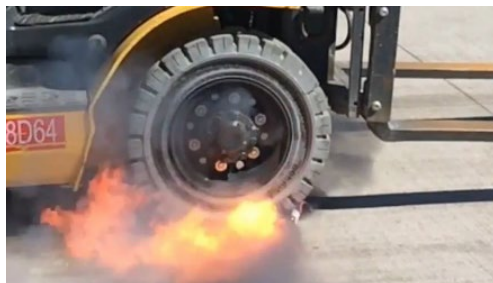
Picture: Demonstration of how easily a fire can be started by being run over by a forklift at a waste facility (Source: ReThinkWaste)
