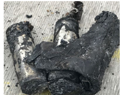
Picture: Burnt batteries from a fire caused by batteries in the recycling stream at the Burbank Recycling Center (Source: City of Burbank)
