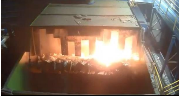
Picture: Fire started by battery improperly disposed in recycling at Shoreway Environmental Center Materials Recovery Facility (Source: ReThinkWaste)
