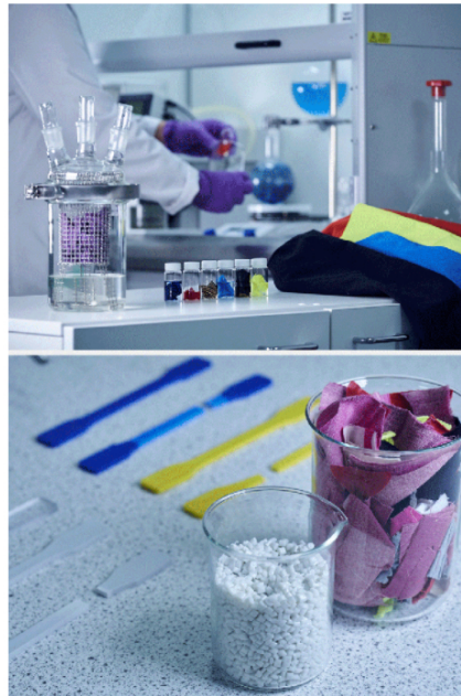
Textile recycling operations at a Worn Again Technologies research lab; process equipment at a UK pilot facility; PET from textile recycling process. © Worn Again Technologies
