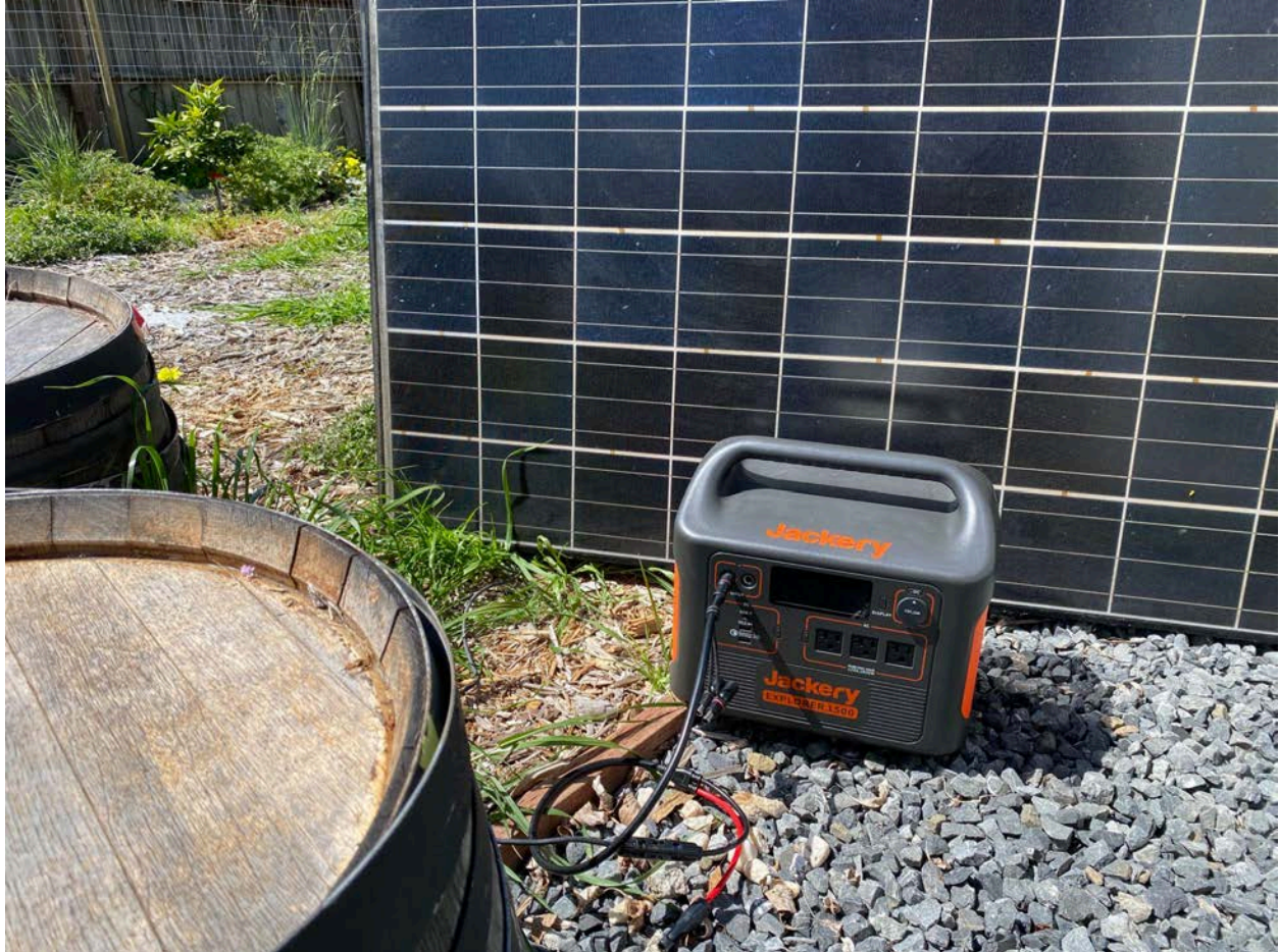
Image 8 : Jackery power station connected to a used solar panel
