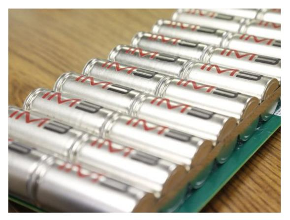
A bank of lithium ion battery cells produced by Charge C4V. (Photo: Patrick Oehler/Staff Photo)
