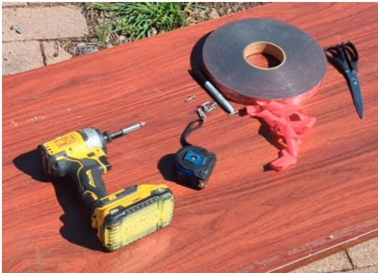
Image 2 : VHB adhesive tape and other tools used.
