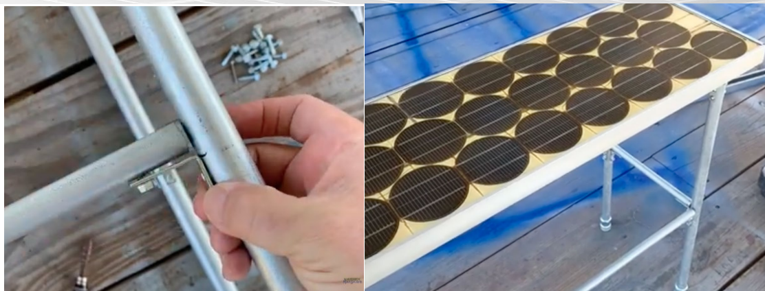
Image above shows how to make table legs out of conduit (image credit and full video: https://www.youtube.com/watch?v=cTijdfHAz2k )
