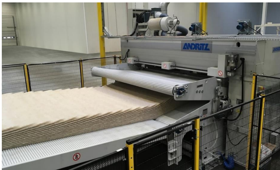
Figure 11: Airlay line Flexiloft by Laroche (Laroche, 2021a)
